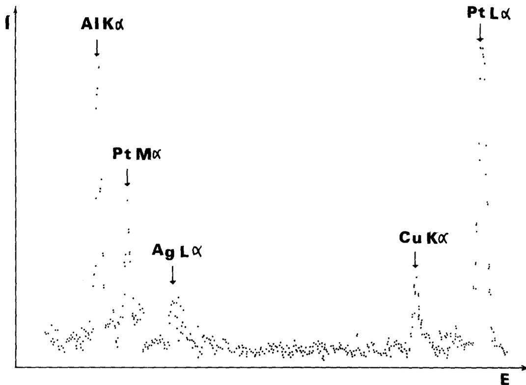
Figure 14 Energy dispersive X-ray spectrum of a metal rod formed during simultaneous colouring with copper and silver near the oxide-metal boundary; the sample holder was platinum.
