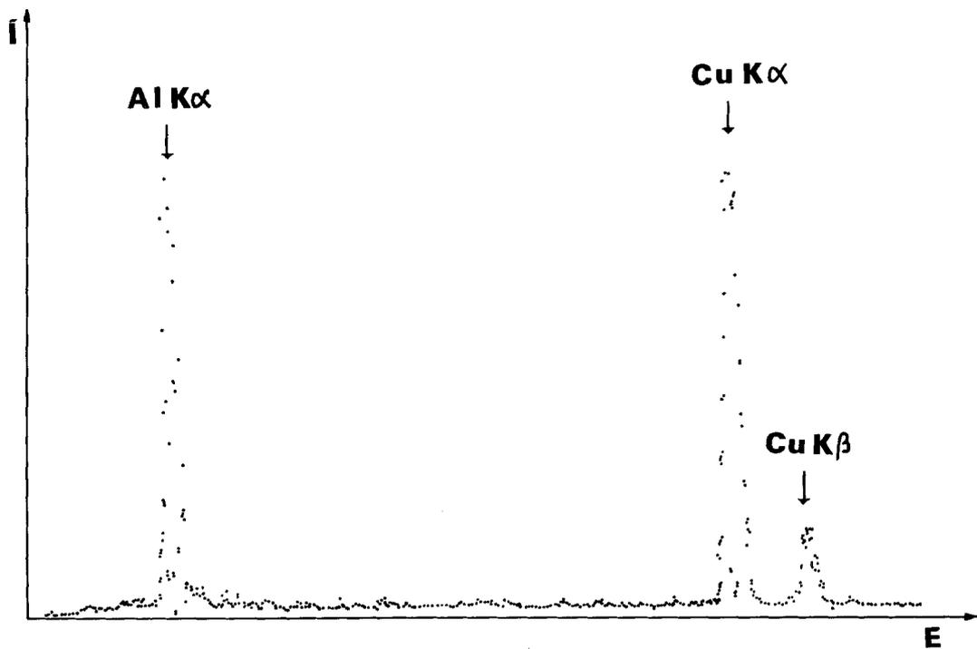
Figure 13 Energy dispersive X-ray spectrum of aluminium; the sample holder was copper.
