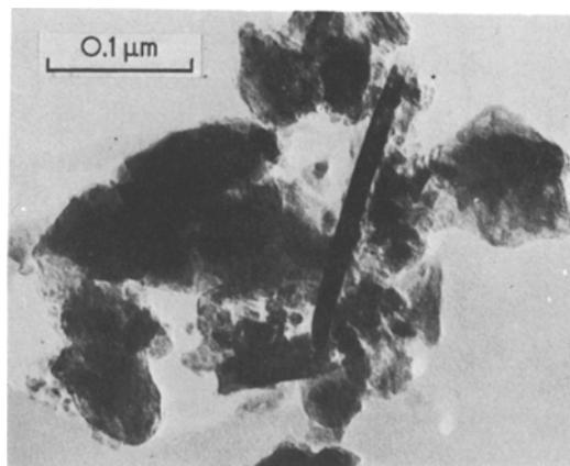
*Figure 11* Transmission electron micrograph of a metal rod found in a specimen crushed in liquid nitrogen.
