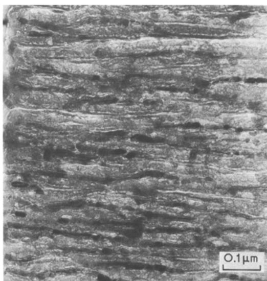
*Figure 10* High magnification transmission electron micrograph of a thin section.
