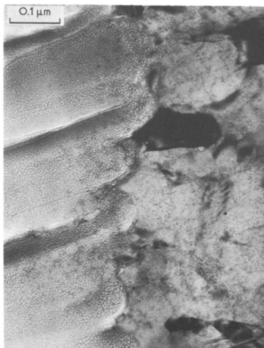
Figure 2 Transmission electron micrograph of an ultra-thin section of an aluminium oxide layer.
