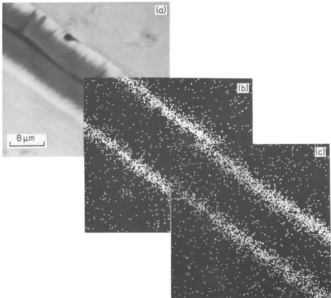
Figure 5 Micrographs made by the electron beam microanalyser on a cross-section of the anodic oxide layer of Sample B (a) backscattered electron picture; (b) X-ray picture of the primary deposited metal; (c) X-ray picture of the secondary deposited metal.
