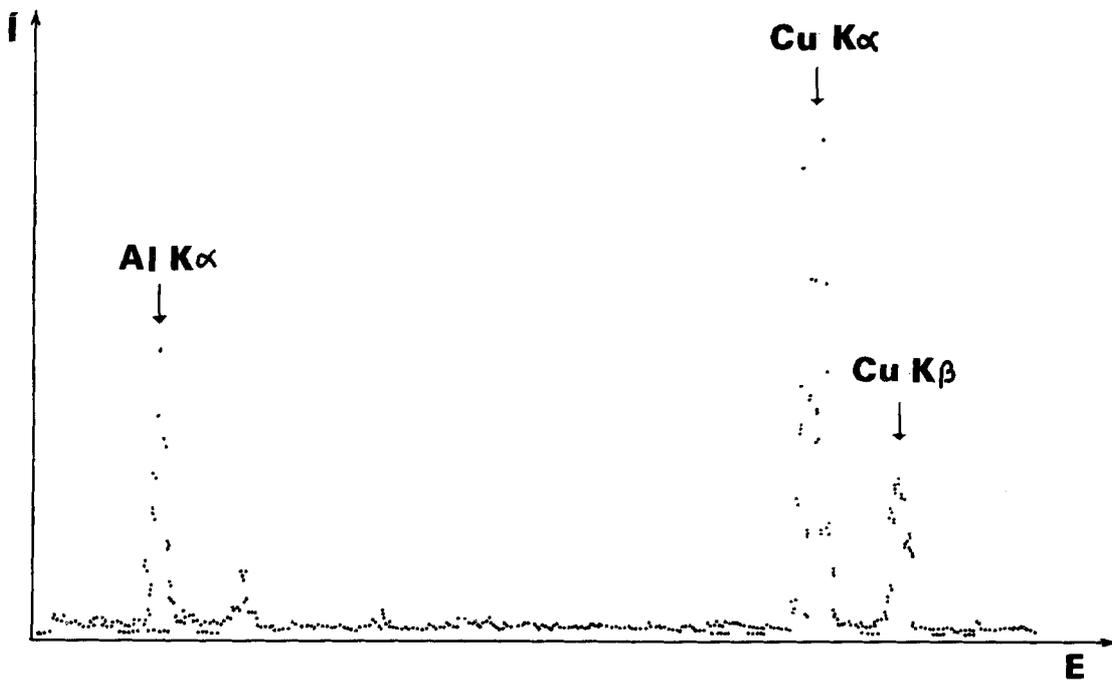
Figure 12 Energy dispersive X-ray spectrum of an anodic aluminium oxide specimen without metal colouring; the sample holder was copper.
