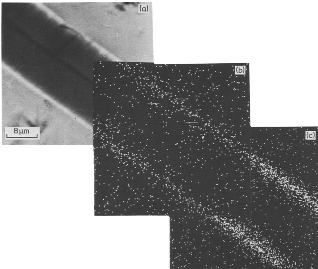
*Figure 3* Micrographs made by the electron beam microanalyser on a cross-section of the simultaneously coloured anodic oxide layer of Sample A (a) backscattered electron picture; (b) X-ray picture of one metal; (c) X-ray picture of the other metal.
