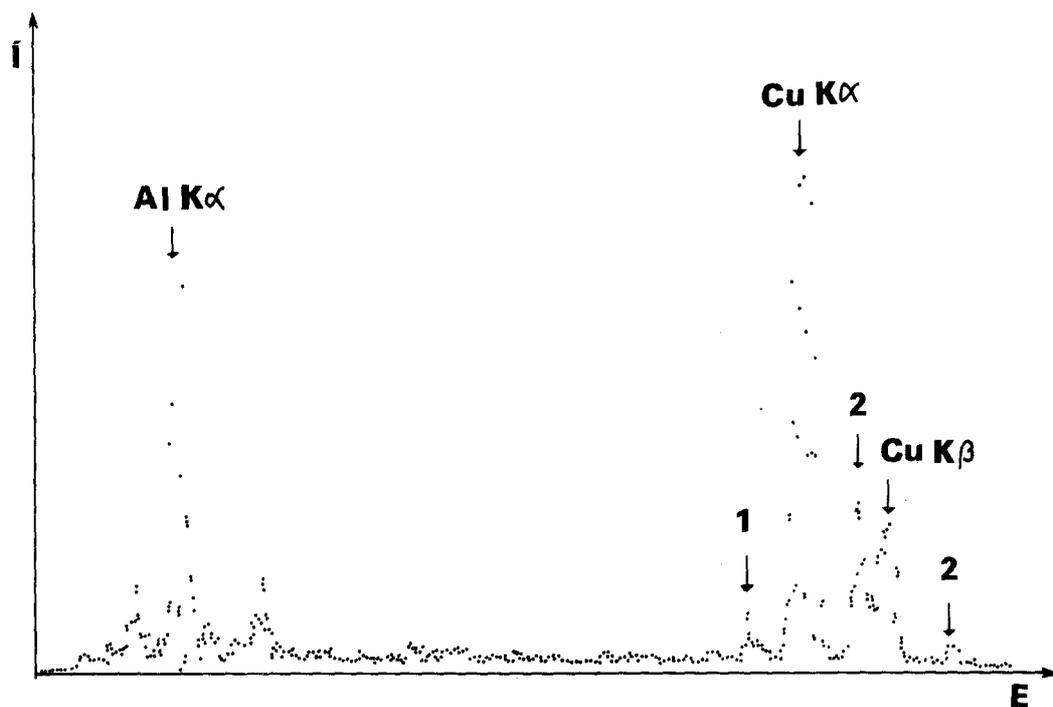
Figure 15 Energy dispersive X-ray spectrum of a metal rod formed during simultaneous colouring with two metals near the oxide-metal boundary in Sample A; the sample holder was copper.
