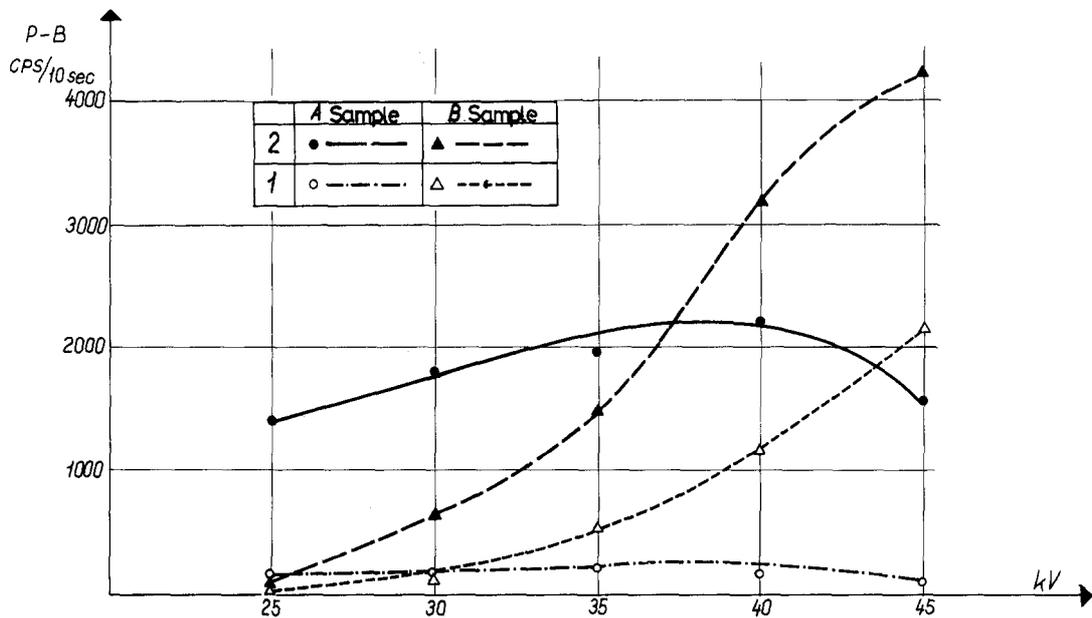
Figure 7 Depth profiling concerning the two metals in the case of Sample A and Sample B from the air-oxide boundary direction.
