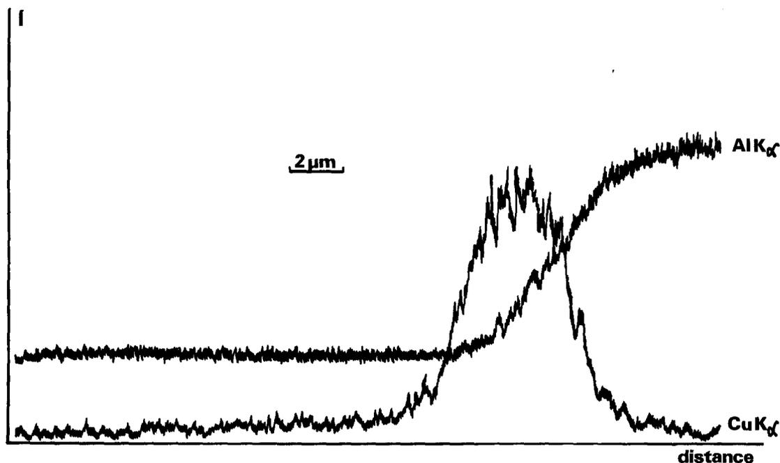
Figure 1 The copper and aluminium line profile of an anodic oxide layer coloured with copper.
